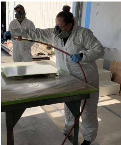
Vanessa Pena applying Gel Coat In the composites unit
